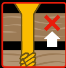
Partially Threaded Stops The Timber Jacking
