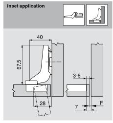
Reset fixing position of mounting plate to door thickness + 1.5 mm
